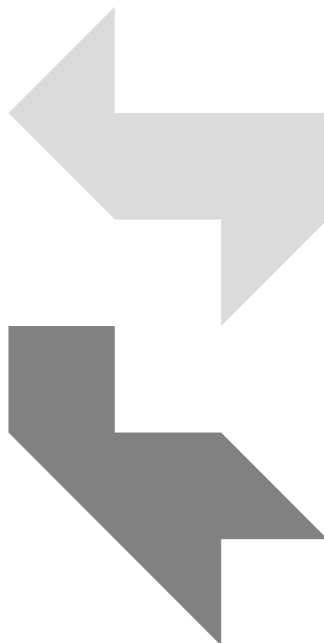
Figure 1 Two isospectral domains in \mathbb{R}^2 whose Laplacians have the same spectrum [14].
